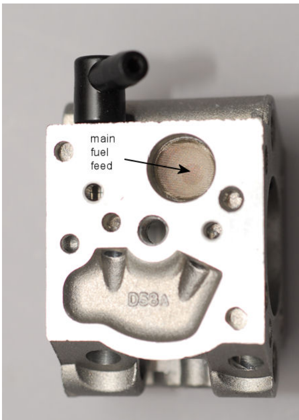
Fuel Path through pump
